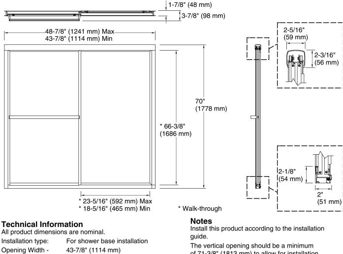
of 71-3/8" (1813 mm) to allow for installation clearance.
